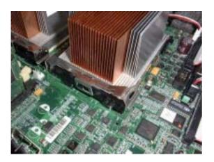
4. Position the heat sink on the processor and hook it on one side of the retention module.
